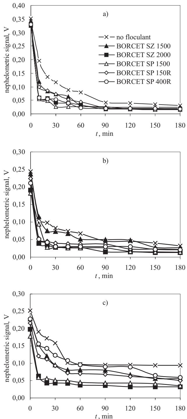
**Fig. 1.** Changes of nephelometric signal in time for suspensions of  $4 \text{ g/dm}^3$  concentration of kaolin (a), bentonite (b) and natural clay (c) without flocculant and in the presence of various flocculants with dose of  $10 \text{ mg/dm}^3$
