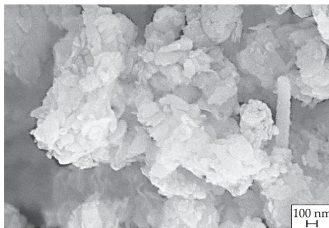
Fig. 1. Microscopic image of halloysite
