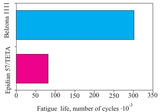
Fig. 7. Comparison of fatigue life of single-lap joints, made with Epidian 57/TETA and Belzona 1111, with the maximum load of fatigue cycle equal to 0.6 of the destructive force
