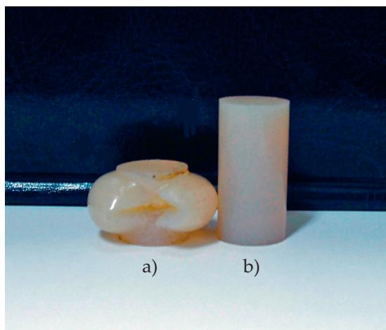
Fig. 1. The strain of a specimen cast from Epidian 57/TETA hardened in the ambient temperature after 30 min of load (30 MPa) in the temp. of 60 °C: a) the specimen after investigation; b) the specimen before investigation
