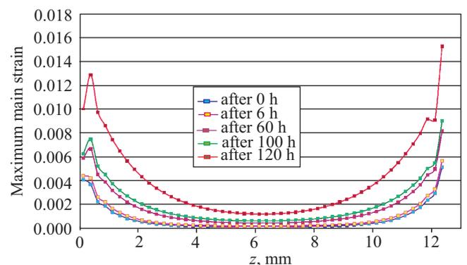
Fig. 13. A change in time of the maximum main strain along (z) the adhesive joint for Belzona 1111
