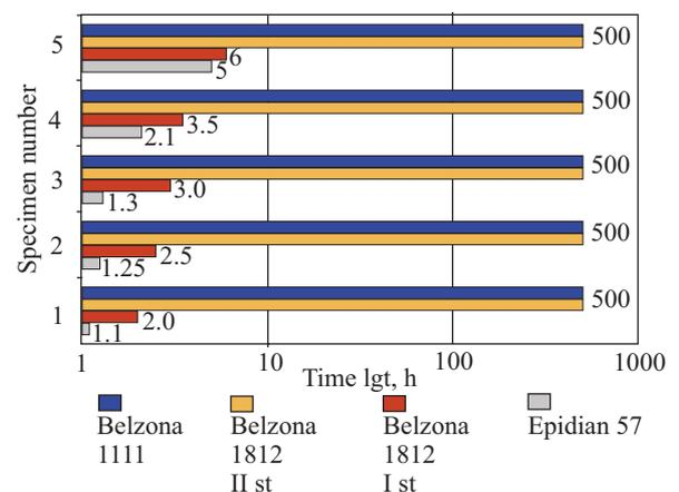
Fig. 5. Static temporal durability of a lap joint made using the investigated adhesive materials (loaded with 60 % of destructive force in the temperature of 60 °C)
