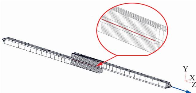
Fig. 10. The discrete model of the adhesive shear loaded lap joint
