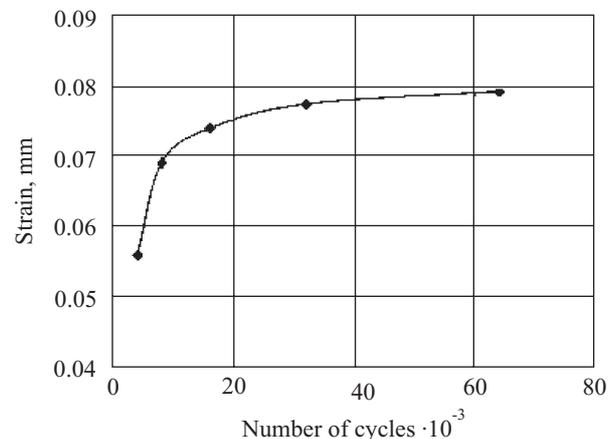
Fig. 8. The change in the scope of strains in a fatigue loaded lap joint in the initial phase of the fatigue investigation [2]
