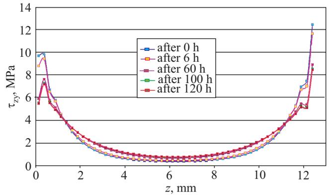
Fig. 11. A change in time of tangential stresses ( $\tau_{zy}$ ) along (z) the adhesive joint for Belzona 1111
