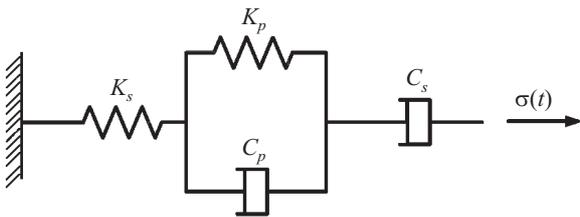
Fig. 9. Model of physical properties of adhesive joint's material used in NASTRAN program to calculate the creep phenomenon
