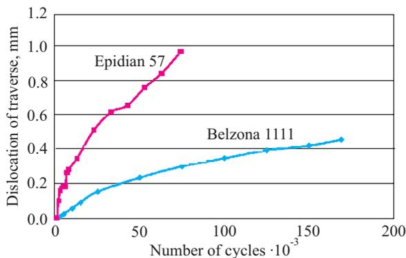
Fig. 6. Dislocations of the traverse head (a change of the specimen's height) depending on the number of cycles for Epidain 57 and Belzona 1111 adhesive materials
