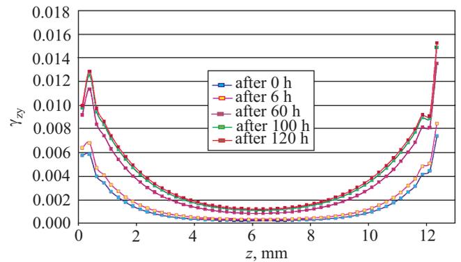
Fig. 12. A change in time of non-dilatational strain in ( $\gamma_{zy}$ ) along (z) the adhesive joint for Belzona 1111
