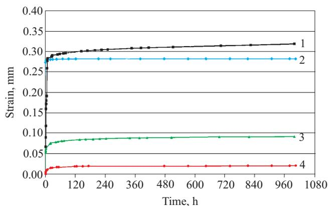
Fig. 3. The creep curves of adhesive materials determined in the temperature of 60 °C for a load that caused normal negative stresses of 30 MPa in the investigated specimens. 1 – Epidian 57, two-stage hardening, 2 – Belzona 1812, single-stage hardening, 3 – Belzona 1111, two-stage hardening, 4 – Belzona 1812, two-stage hardening
