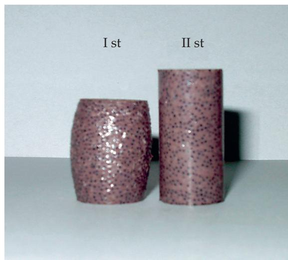
Fig. 2. The comparison of stains of specimens cast from Belzona 1812 composite (single-stage hardening – I st and two-stage hardening – II st), investigated in the temperature of 60 °C under load, which caused normal negative stresses of 30 MPa
