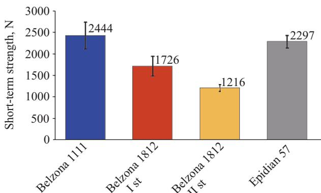
Fig. 4. Short-term strength of lap joints made using investigated adhesive materials (single-stage hardening – I st and two-stage hardening – II st)
