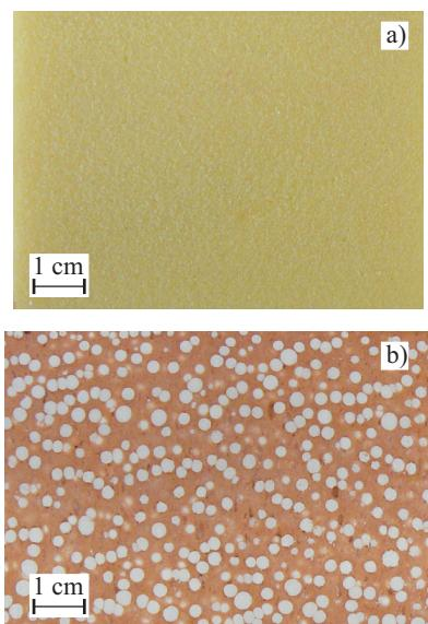
Fig. 1. The cross-section appearance of foam samples:
