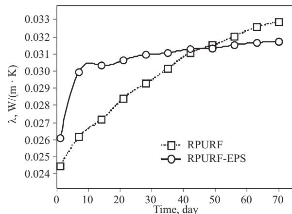
Fig. 2. Effect of the ageing time on thermal conductivity for reference RPURF and RPURF-EPS composite samples
